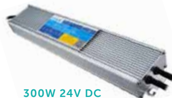
300W 24V DC LED Power Supply Model: APS-300-24A Input: 100~277V AC Output: 24V DC 12.5A
